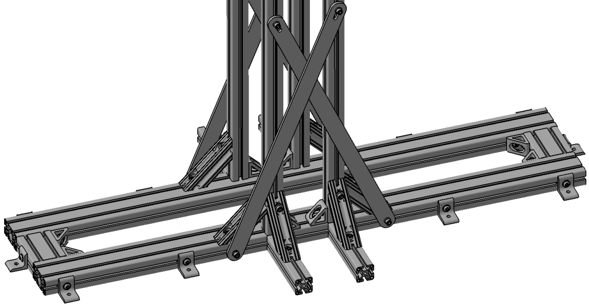
Fig. 4.21: Coaxial assembled support: base section
