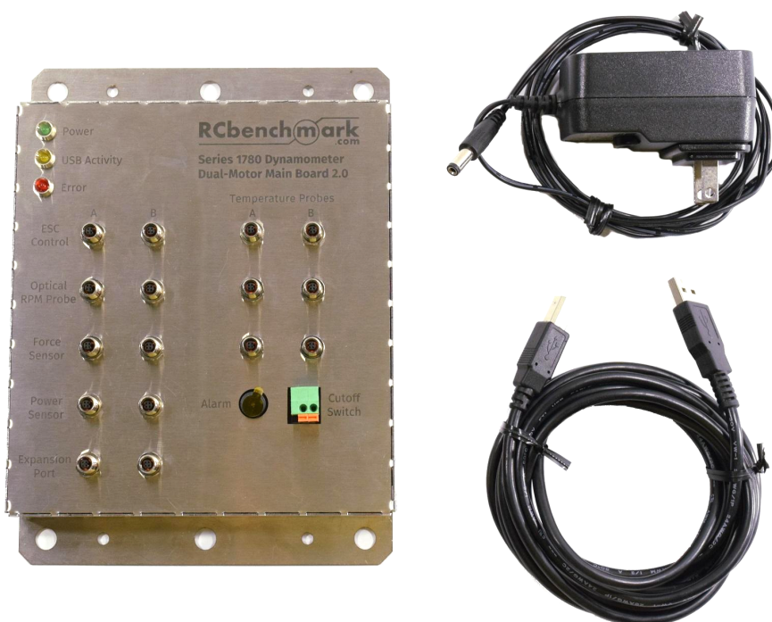
Fig. 4.43: Photo of dual main board with USB cable and power adapter
