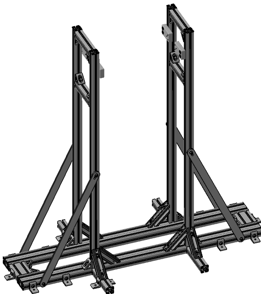
Fig. 4.26: Assembled support for coaxial face-to-face setup
