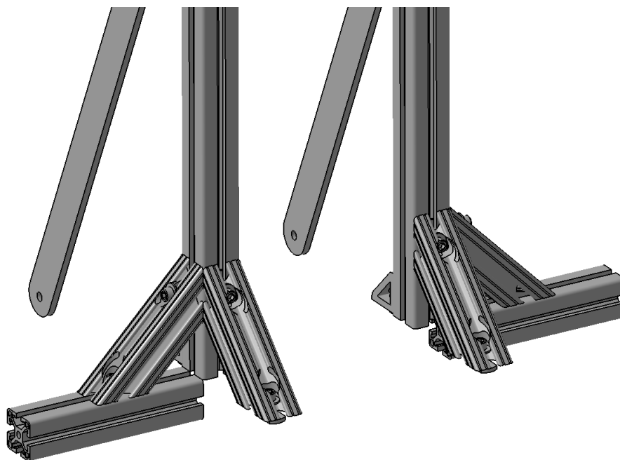
Fig. 4.14: Diagonal beam 6" (#QFGJ) attached to the T-slotted frame 4" (#HJXQ) and 7" (#NWGF)
