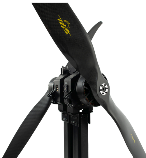
Figure 25: Flight Stand 150 thrust stand in a coaxial set-up
