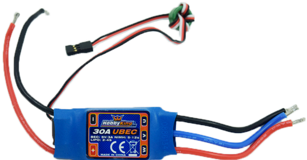
Figure 17: External view of ESC wiring
