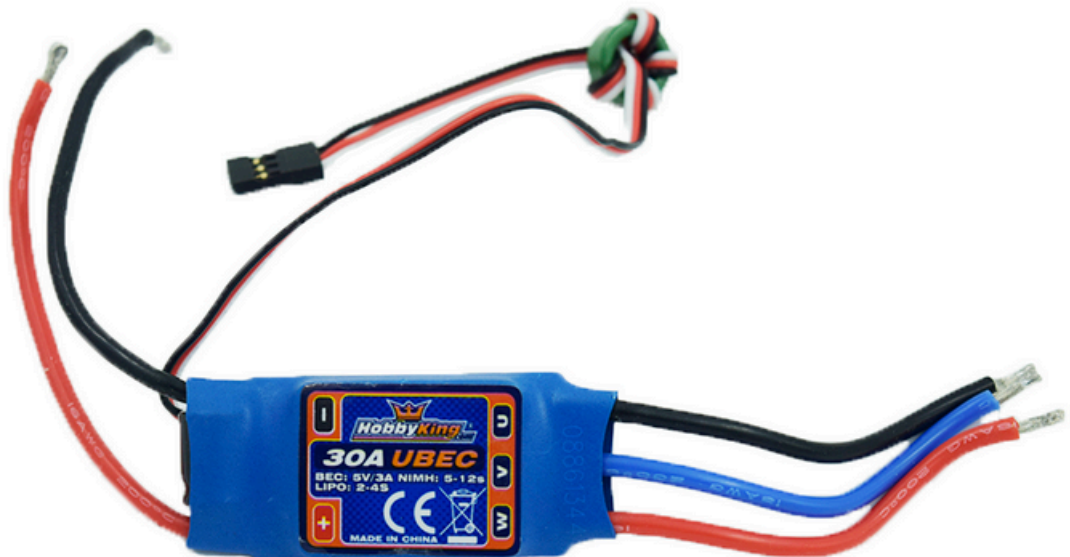
Figure 17: External view of ESC wiring
