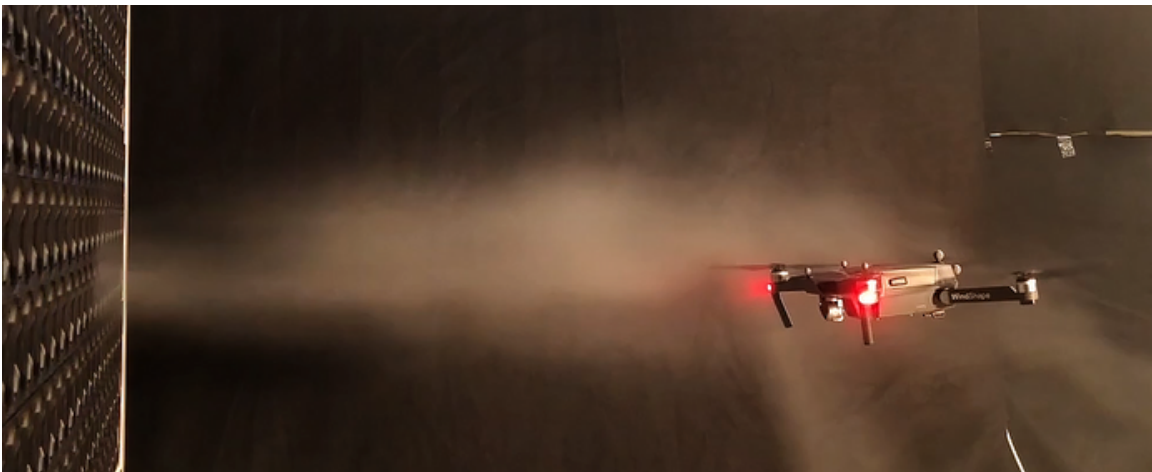
Figure 29: Testing a drone in rain and fog ( click for video )
