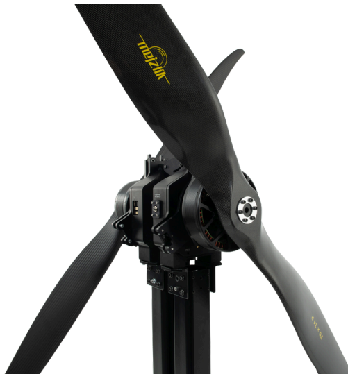
Figure 24: Flight Stand 150 thrust stand in a coaxial set-up
